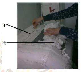
Sampling process Figure determining fine impurities in raw cotton in the laboratory.
