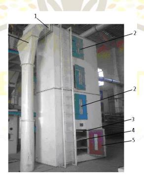
Figure 1: Overview of a tower dryer
