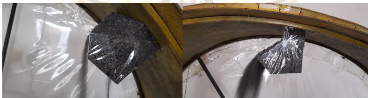
Figure-3. processes of mineral fertilizer spillage from the nozzle
