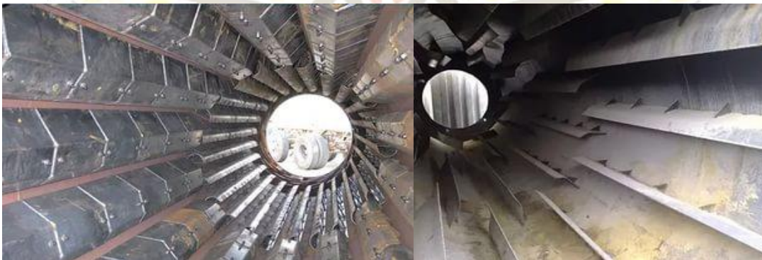
Figure 1. The structure of Nozzles in the drum
