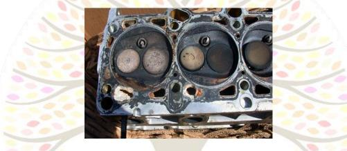
Figure 1. Engine burns due to overheating
