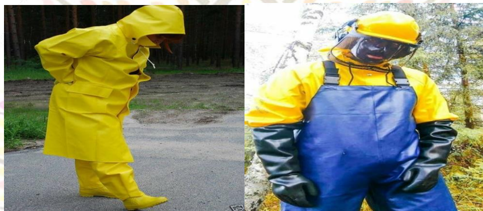
Figure 3. Clothes welded with the high-frequency current.
