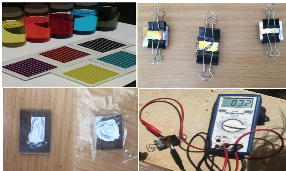
Figure 2. Measurement of the voltage and current values of solar cells based on photosensitive dyes and the power they produce
