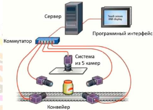
Fig. 4. System of 5 cameras for quality control of products on the conveyor
