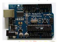
Fig. 1. Microcontroller Arduino UNO.
