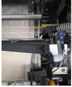
Figure 3. False edge formation on the machine
