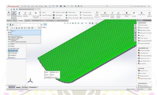
Figure 4. Area of the mesh surface at an angle  $\alpha 1=900$  relative to the center of the spiked drum
