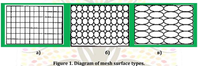
a). woven from steel wire. b), c). made of sheet metal with various holes..
