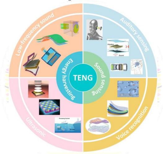
Advances in triboelectric nanogenerators in acoustics: Energy harvesting and Sound sensing
