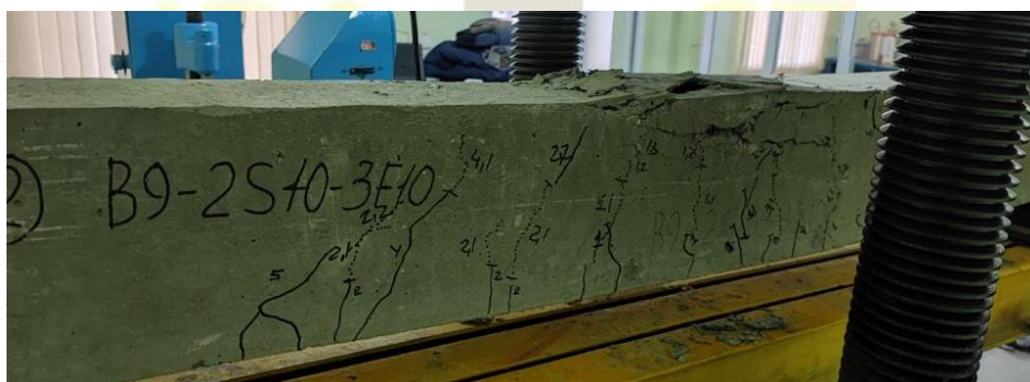
Fig. 6. Failure modes of beams under applied loading
