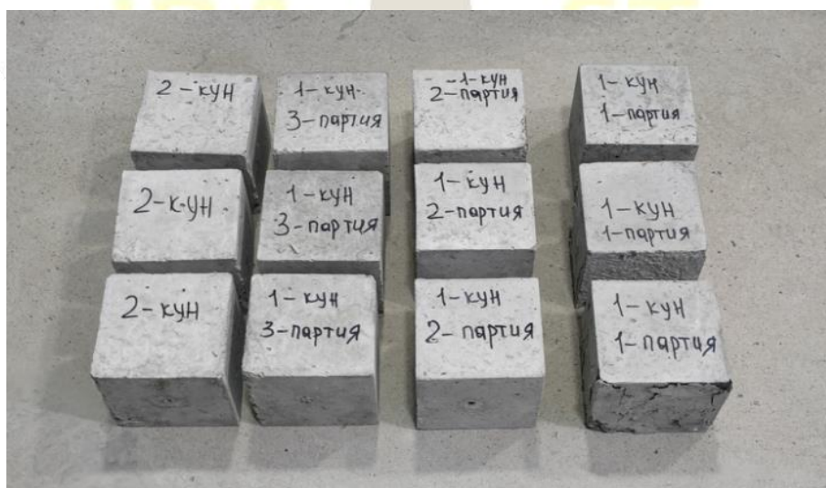
Fig. 3. Prepared cube specimens
