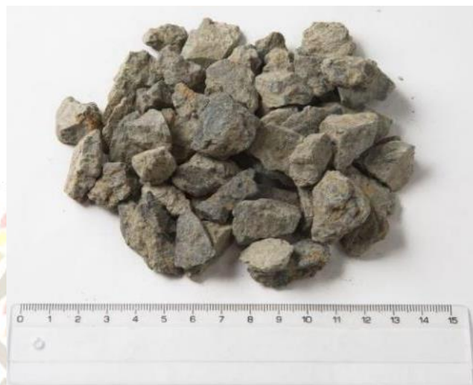
Fig. 2. Crushed stone used for the concrete mix
