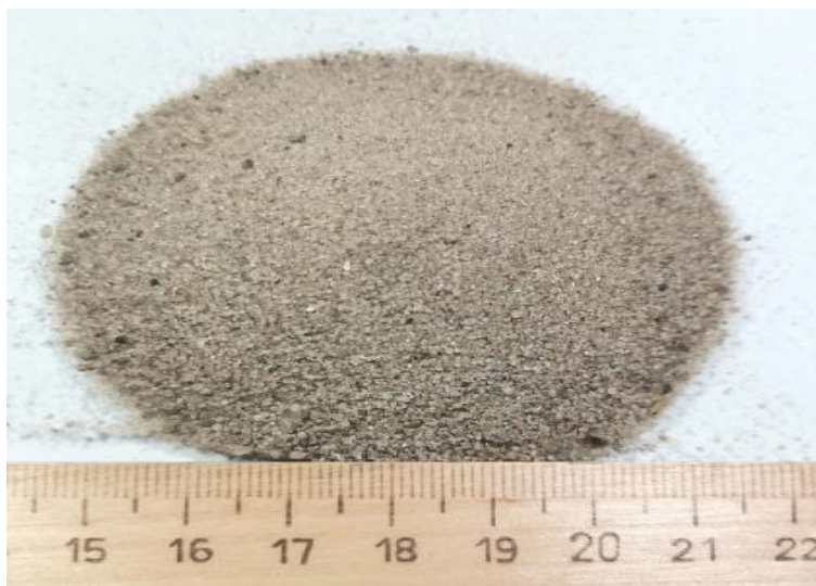
Fig. 1. Sand used for the concrete mix
