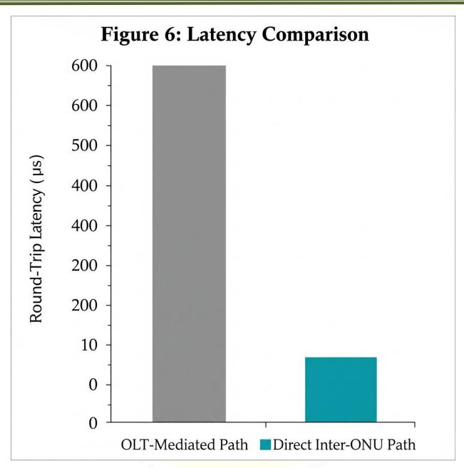
As shown in Figure 6, the results confirm a substantial latency reduction. The direct inter-ONU link consistently demonstrates an RTT that is significantly lower than the OLT-mediated path. The exact reduction depends on the physical location of the OLT relative to the ONUs, but for a
