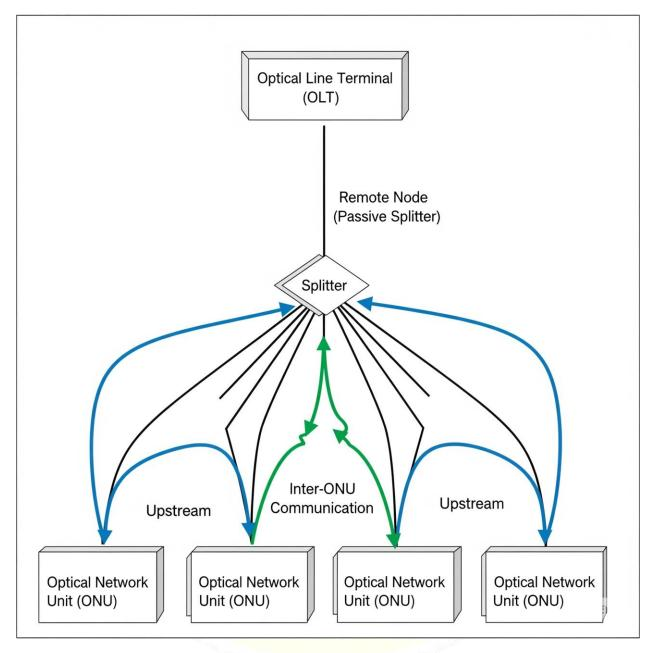
The network architecture under investigation, illustrated in Figure 1, is an IMDD PON designed to leverage the unique capabilities of P2MP flexible optical transceivers. The architecture consists of three primary components: a single OLT located at the central office, a completely
