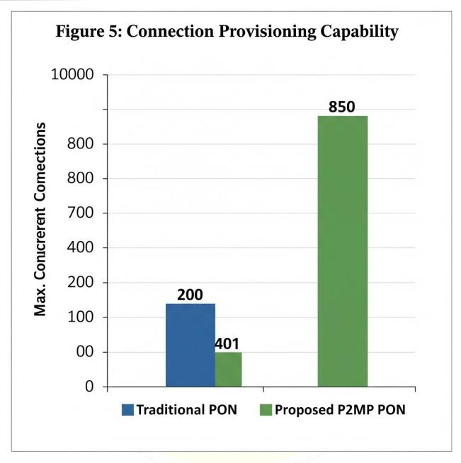
Figure 5 presents the key results of this analysis. It plots the connection provisioning capability of the proposed system against that of a traditional TDM-PON, where all inter-ONU traffic must be routed through the OLT. The proposed system, with its ability for direct ONU-to-ONU
