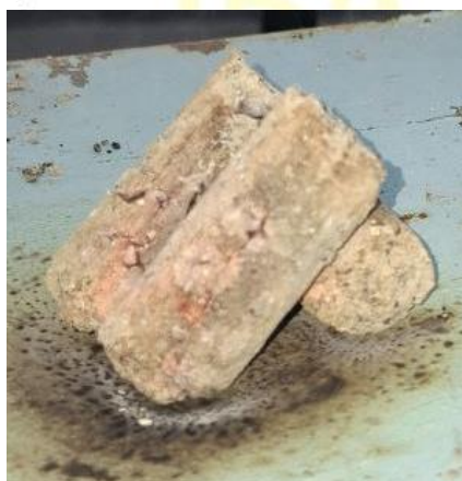
Figure 4a. Initial glowing stage of the coal briquette.
