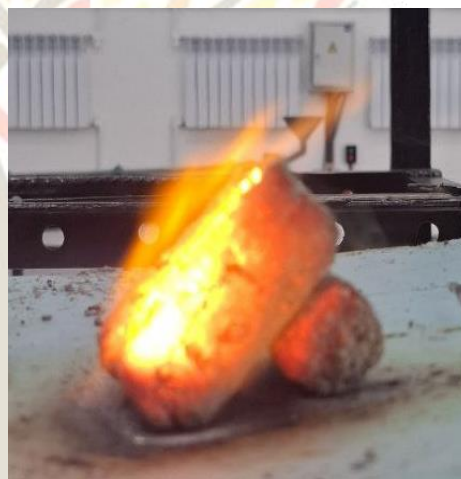
Figure 4b. Full glowing stage of the coal briquette.
