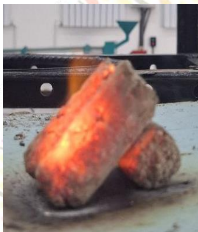
Figure 4a. Initial glowing stage of the coal briquette.
